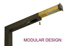
The PL-15 path light is available in aluminum or brass square tubing. The components that house and seal the lamp are machined from copper-free aluminum, then anodized to prevent corrosion from all types of elements. Stainless steel hardware and silicone o-ring seals are standard features. To relamp this luminaire, simply remove one screw and slide out the lamp housing.
